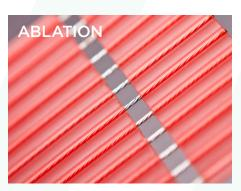
Optimized wavelengths and excellent poser stability allow precise removal of insulation and coatings without damaging the underlying materials.
