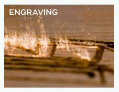
The high peak power is essential to minimizing heat build-up and avoid cracking when processing brittle materials such as alumina, ceramic and quartz glass. Excellent beam quality allows for very small features and clean symmetric holes.
