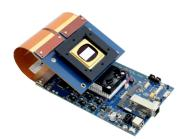
High-performance DLP (Digital Light Processing) from Texas Instrument is a technology of MEMS spatial light modulators that goes far beyond standard multimedia projections and automotive display applications.
