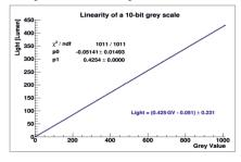
ALP-4 supports precise bit-plane timing enabling outstanding greyscale linearity in connection with synchronized camera recording.
