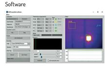
Acquisition Software - Visualization Software - Black hot / White hot spots Image histogram - Store & analyze digital images / movies Image live view - False color mode with various color profiles Spot meters, time profiles - Thermography - Alarms
