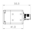
LIR320 is a SWaP-C camera (small size, weight, power and cost). Its dimensions are  $28.5 \times 28.5 \times 55.5$  mm and its weight is lower than 70 grams.
